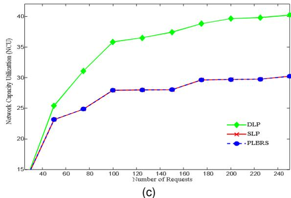
**Fig. 4** (a) Shows Network Capacity Utilization vs. Number of requests for COST 239 and (b) represents the Network capacity utilization vs. Number of requests for ARPANET (c) shows the Network capacity utilization vs. Number of requests for NSFNET.
