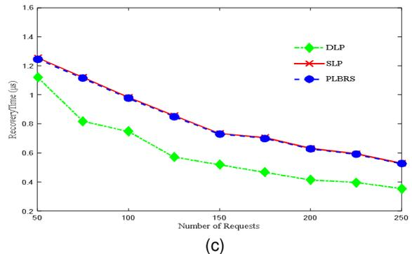
**Fig. 5** (a) Shows Recovery Time vs. Number of Requests for COST 239 and (b) represents the Recovery Time vs. Number of requests for ARPANET (c) shows the Recovery Time vs. Number of requests for NSFNET.
