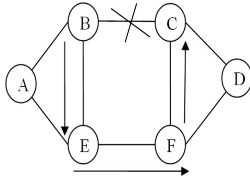
**Fig. 1.** An example of proposed link based recovery scheme (PLBRS).
