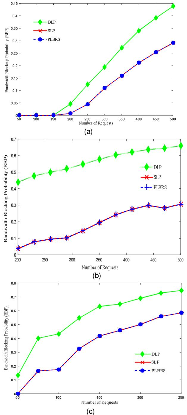
**Fig. 3** (a) Shows Bandwidth Blocking Probability vs. Number of requests for COST 239 and (b) represents the Bandwidth blocking probability vs. Number of requests for ARPANET (c) shows the Bandwidth blocking probability vs. Number of requests for NSFNET.
